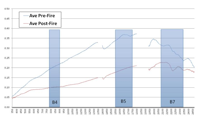
Figure 3: Pre- and Post-Fire average spectral profiles of an arid village. ETM+ bands 4, 5, and 7 are shown (US Geological Society, 2011). The water absorption bands from 1350um to 1400um and 1800um to 1900um are omitted.
